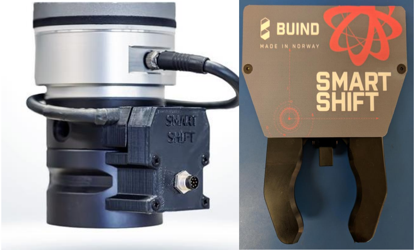
Pic. 01 SMARTSHIFT Electrical & Pneumatic Robot Master (RM) connected to Tool Holder (TH) Pic. 02 Tool Gripper (TG)
